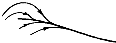
FIGURE 10. Sketch of open separation.
